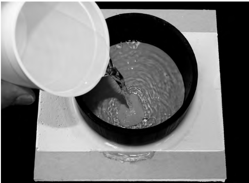
Figure 3: Setup to measure water uptake (Cobb-test).
