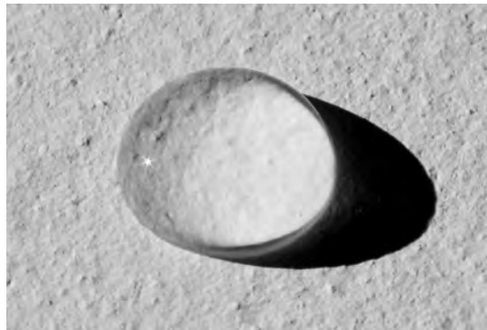
Figure 12: Water drop on surface of gypsum based joint filler modified with Elotex experimental hydrophobizing additive for neutral pH.
